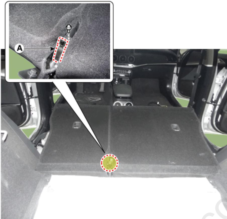
7. Remove the rear seat back assembly (A).
